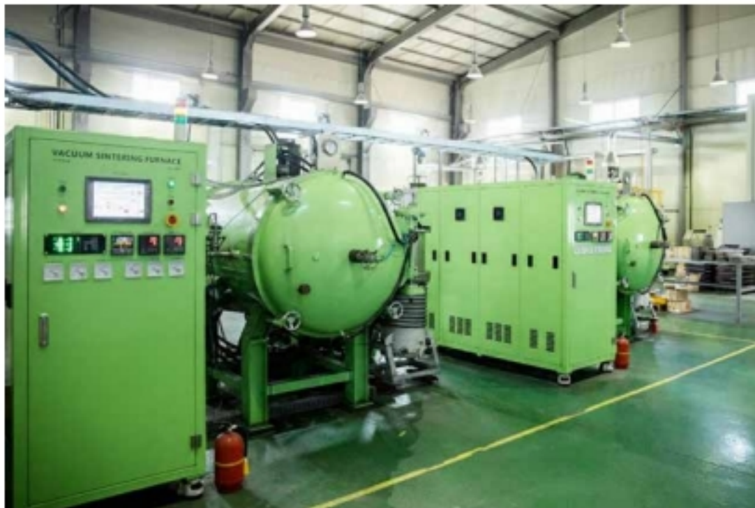
Fig. 3 Vacuum sintering furnaces at MTIG's Hwaseong plant used for densification of titanium MIM parts (Courtesy MTIG)
